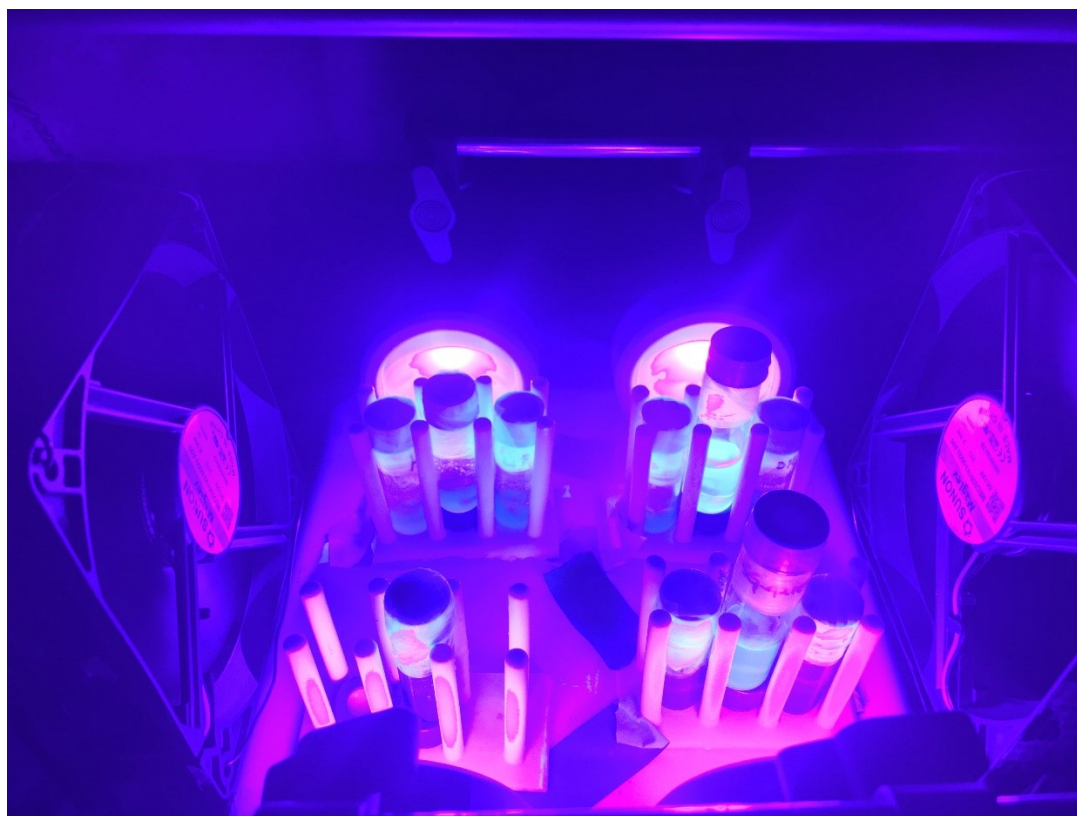
Figure S1. Model Reaction Setup for the Photochemical Arylation on Acrylamides
