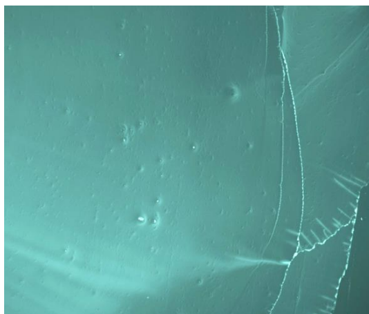
Figure S13. Fluorescence image showing the morphology of the thin film obtained by the solvent evaporation of the chloroform solution of P6 on a silicon wafer. Solution concentration: 0.1 mg/mL.
