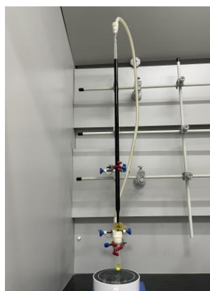
Supplementary Fig. 1 Digital photo of titration set-up by Karl Fischer reagent.
