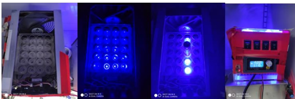
Figure S1. Set-up for photoredox reactions
