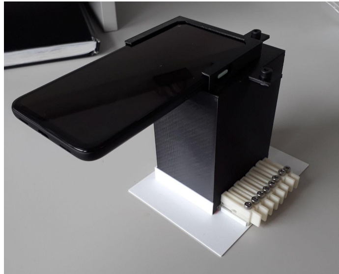
Fig. S1: Photograph of the modular setup with the mounted smartphone and eight strips inserted.
