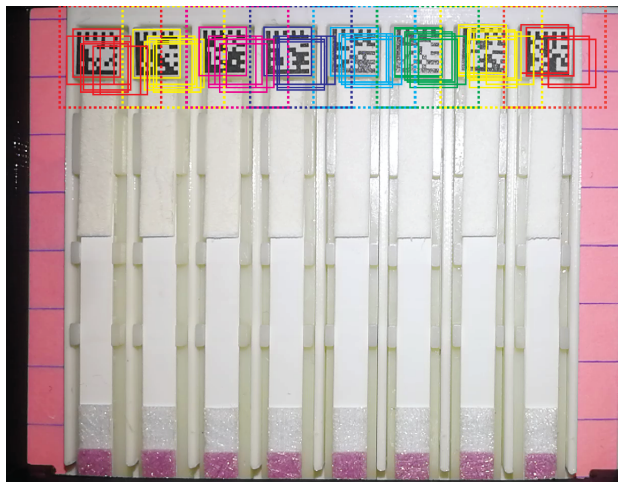
Fig. S10: Variation in strip positions on the different lanes. The variation stems from slight differences in smartphone positioning and is compensated by the app by calculating the various regions relative to the position of the detected QR codes.
