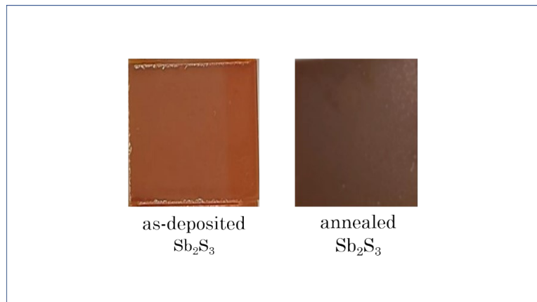
Figure S2: \text{Sb}_2\text{S}_3 films undergo a change in color from light brown in as deposited state to dark brown post annealing. Substrate: glass/FTO/ \text{TiO}_2 .
