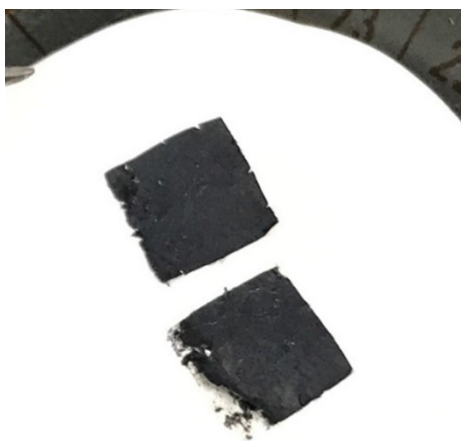
Figure S3. Photograph of CNT/PBI/Pt films fabricated using probe sonication in the preparation step.
