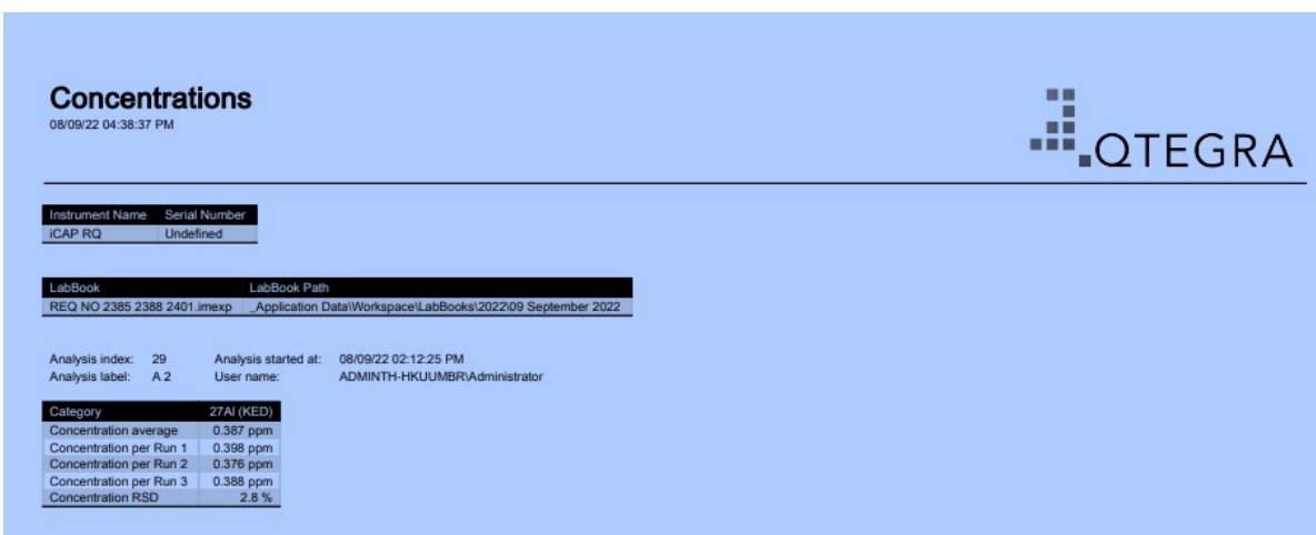
Figure S2. The amount of Al in \text{Al}_2\text{O}_3 -rGO nanocomposite materials as determined by ICP-MS. The result shows that the amount of Al on rGO surface is 2.8 wt.%.
