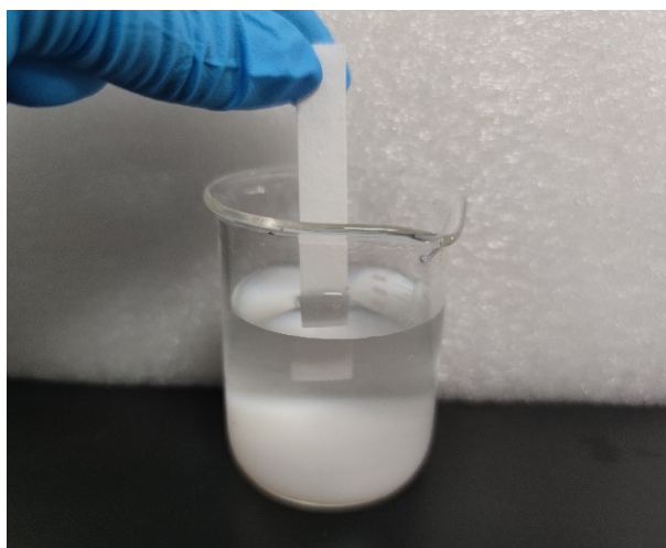
Fig. S14. The digital photograph of the results for ClO - formation in 1 M KOH seawater electrolyte after OER stability testing of NiMoO 4 @NiFe LDH at 100 mA cm -2 for 80 h. The formation of hypochlorite (ClO - ) was examined via the potassium iodide starch paper.
