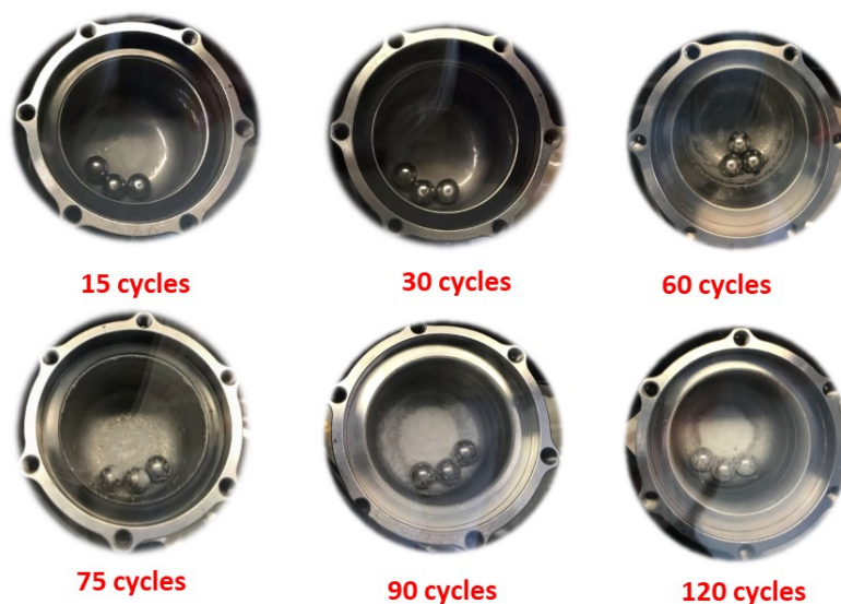
Fig. S7 Photographs of product after different amounts of milling cycles based on Approach A.
