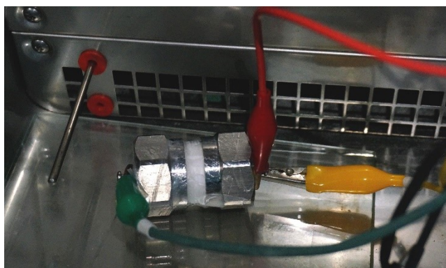
Figure S4. The picture of a Swagelok symmetric cell with two stainless-steel rods.
