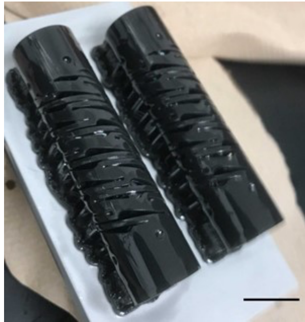
Figure S1. Photograph of two 1x HSAs immediately after printing. Scale bar represents 20 mm.
