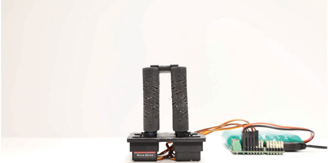
Movie S1. Multi-DOF actuations of the 0.5x HSA Leg (stills are shown in Fig. 4b).
