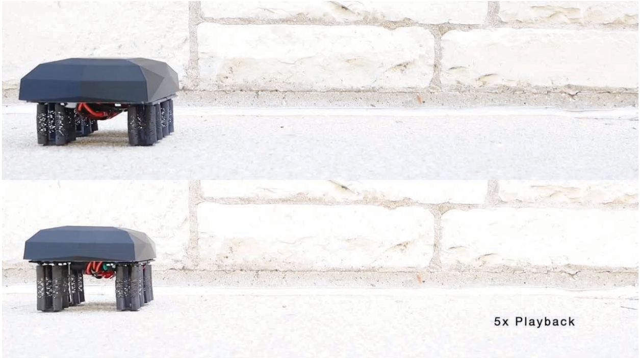
Movie S4. Untethered soft robots walking on concrete sidewalk. The top and bottom clips show the quadrupeds constructed from the 0.5x Legs and Stilted 0.5x Legs, respectively. Video playback is 5x.
