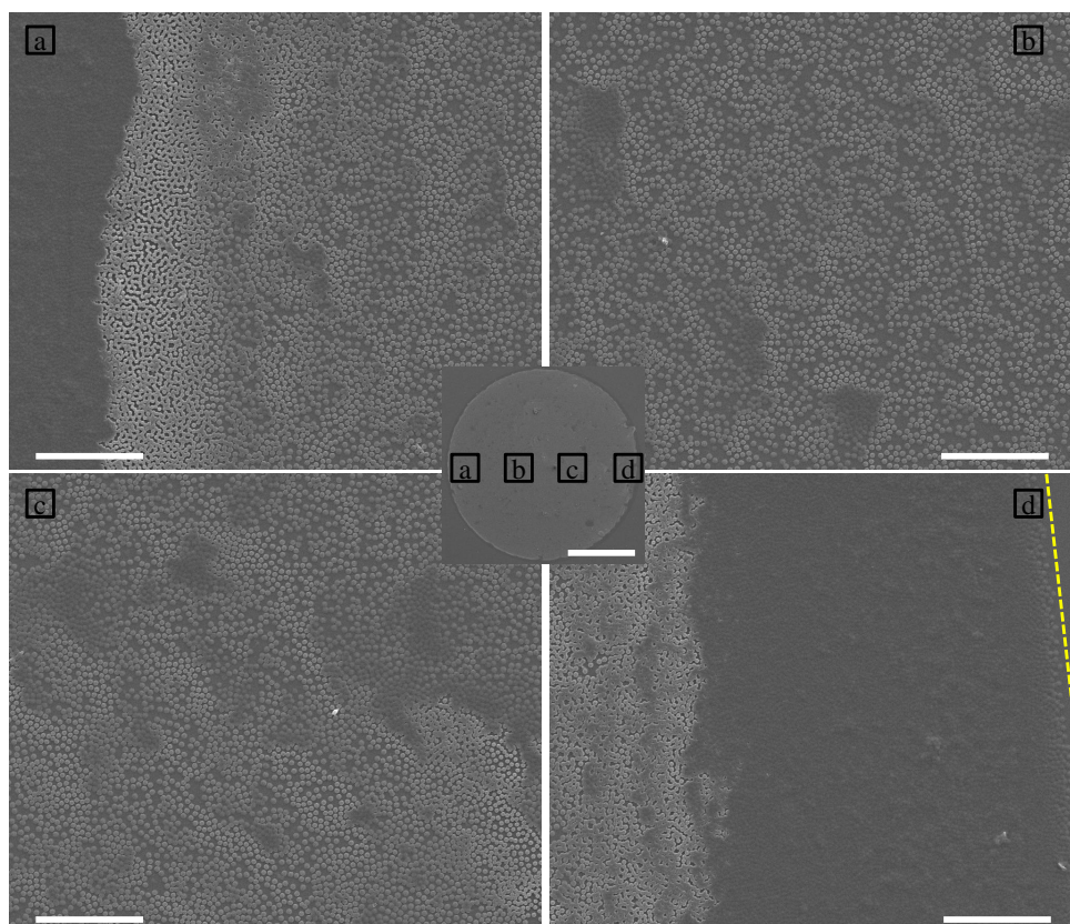
Figure S5: SEM images of the particulate deposit formed by the p-NIPAM microgel particles on the hydrophobic substrate at different regions marked a), b), c) and d) in the central low magnification image. Microgels at different levels of compression can be seen at different regions of the deposit. The yellow dashed line in (d) is drawn to indicate the exterior of the deposit. Near the periphery, the dark regions in the image (a and d) correspond to particles that are highly compressed and probably forming multi-particle layer. Scale bars: 500 \mu\text{m} (central low magnification image) and 10 \mu\text{m} (high magnification images a, b, c and d).
