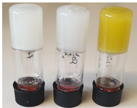
Figure S1. Gels of Palm-Phe in different edible oils at a concentration of 2 wt%. From left to right: rapeseed oil, sunflower oil and olive oil.
