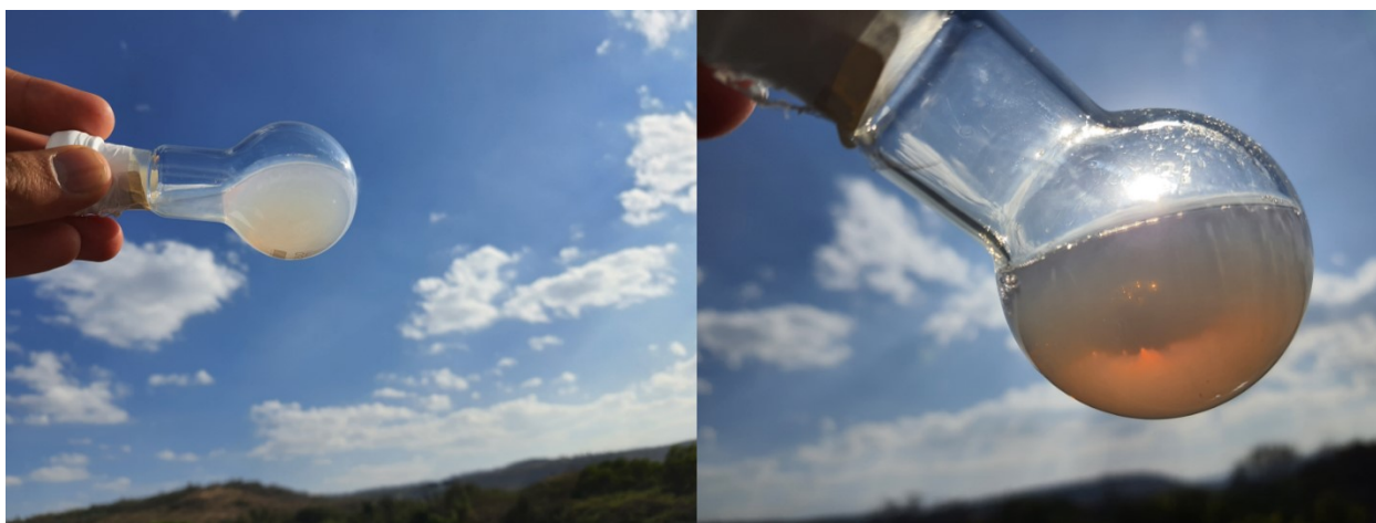
Figure S1: Digital photographs to show an uniform dispersion of the catalyst during reaction under direct sunlight.
