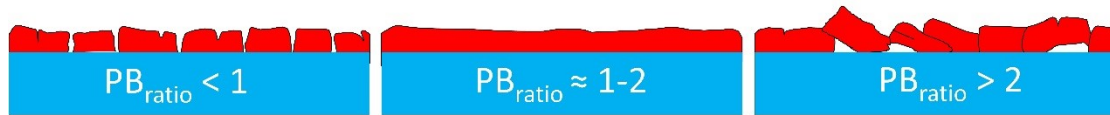
Fig. S4 Schematic diagram of the thin film morphology and the corresponding Pillings-Bedworth ratio.
