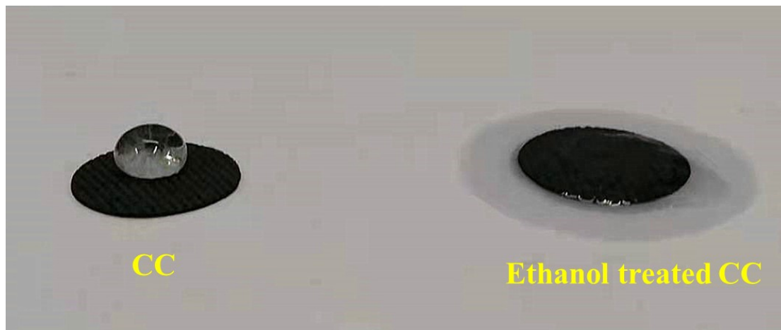
Figure S1. The wetting behavior of aqueous \text{Pb}(\text{Ac})_2 \cdot 3\text{H}_2\text{O} solution on carbon cloth with (left) and without (right) alcohol pre-treatment.
