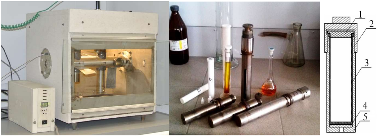
Fig. S1. Photos of autoclave in air heating device (thermostat) along with the components and scheme of the pressure vessel: 1 – Teflon lead, 2 – Ti nut, 3 – Teflon liner, 4 – plate, 5 – Ti base body.
