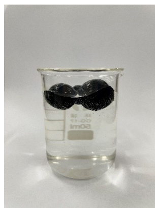
Fig. S8 Photograph of the obtained MF-SA/TA- \text{Fe}^{3+} self-float in water.
