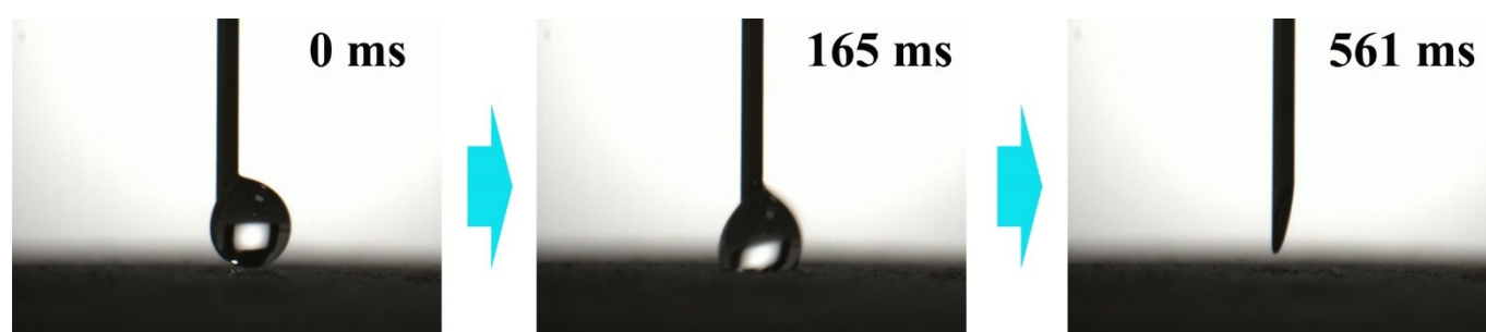
Fig. S5 Water wetting behavior on MF-SA/TA-Fe 3+ surface.
