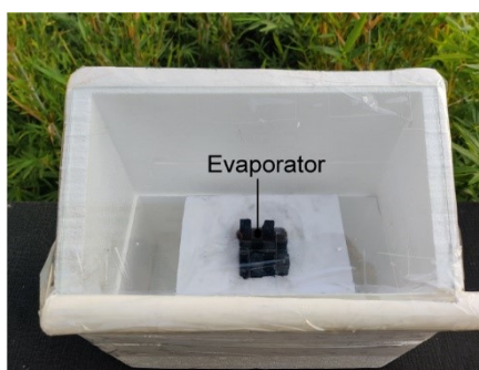
Fig. S9 Photograph of the air cooling-assisted vapor condensation set during outdoor experiment on rooftop at Zijingang campus.
