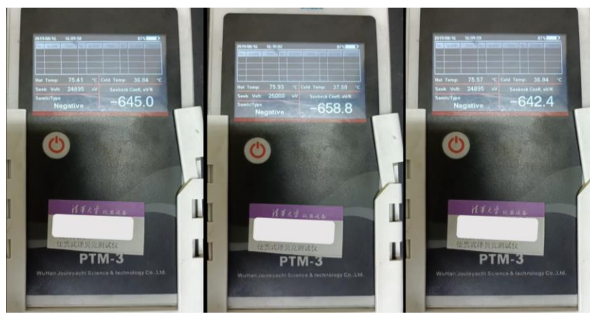
Fig. S7 The Seebeck coefficient testment results of the film surface at 400 °C
