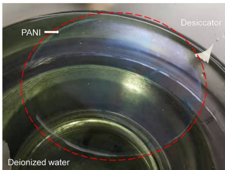
Figure S1. Photograph of the PANI nanoscale thin film on the water interface.
