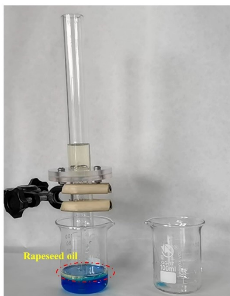
Fig. S11 Oil-water separation test of ordinary glass fiber membrane
