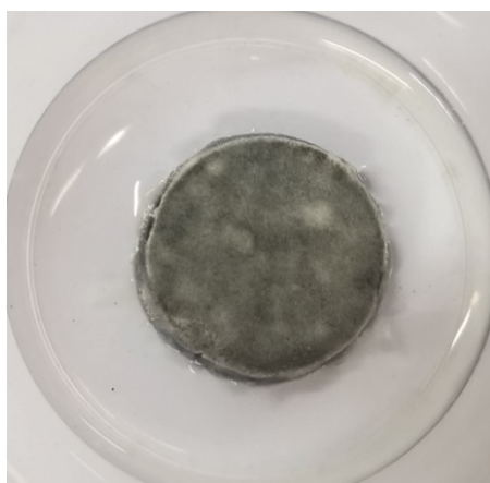
Fig. S11. Photograph of the moldy CDSA.
