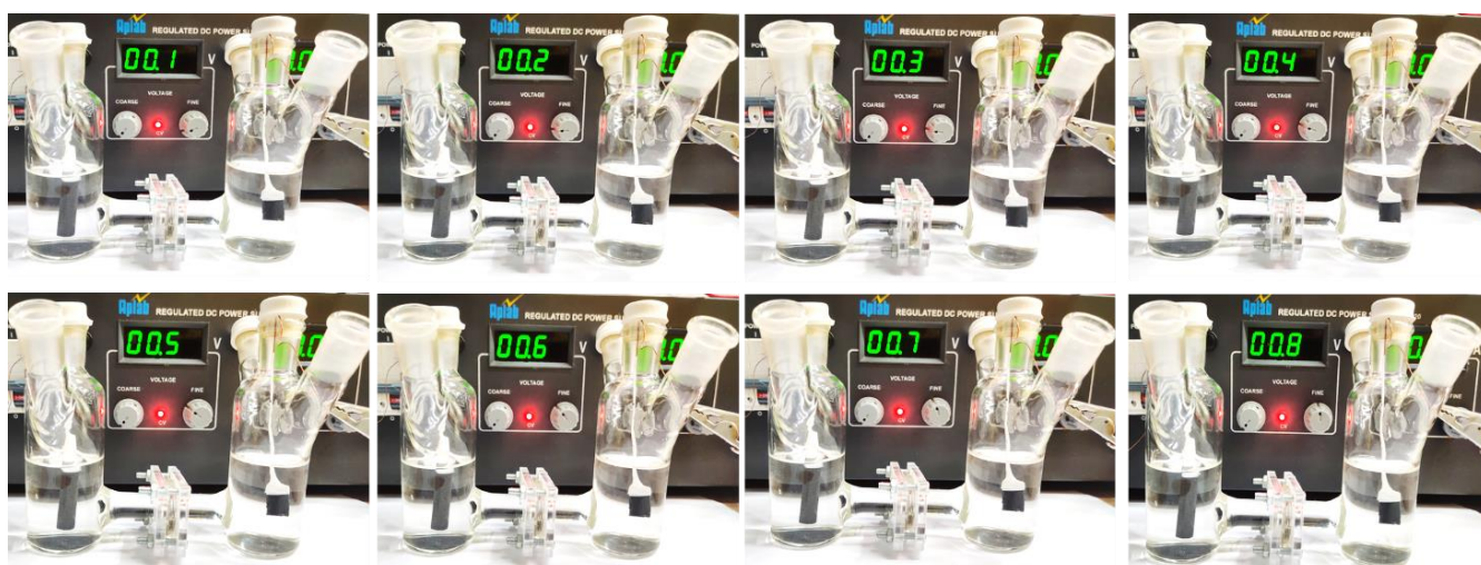
Fig. S33. Photographic images of the device constructed in H cell to drive splitting of \text{H}_2\text{O} in 1 M NaOH at different potentials, using NiCu-MoS 2 coated graphite paper working electrode and graphite counter electrode.
