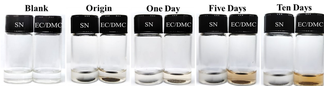
Fig. S9. Visualization dissolution experiment of P5Q in 5 mol% \text{NaClO}_4/\text{SN} PCE and \text{NaClO}_4/\text{EC}+\text{DMC} electrolytes.
