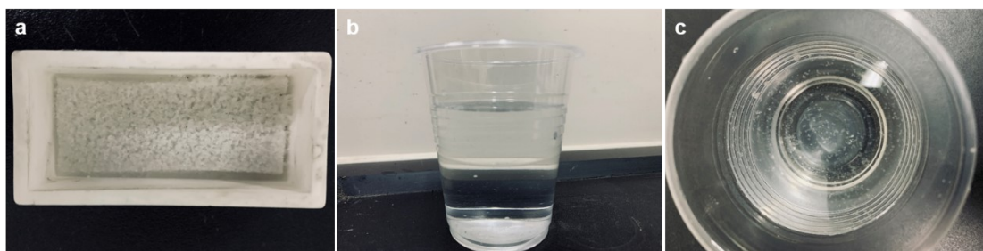
Fig. S7 Images of calcined products of KCl and KSCN: (a) after cooling; (b) and (c) after dissolving in water.
