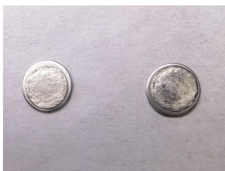
Fig. S10 Photographs of the Li electrodes of the Li|AP-PE|Li (left) and Li|P-PE|Li (right) cells after 500 h cycling at 0.1 \text{ mA cm}^{-2} and 0.1 \text{ mAh cm}^{-2} .
