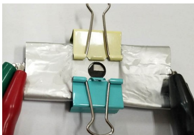
Figure S1. The photo of the solar photothermal solid-state Li-S battery based on the Cu-Si NWs photothermal current collector.
