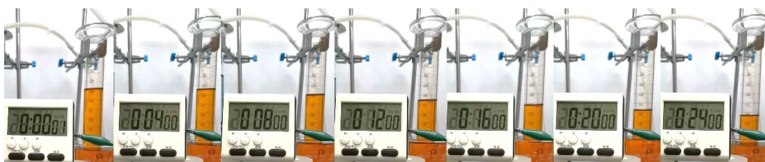
Fig. S27 Digital photograph of a drainage setup for collecting O 2 from water splitting by Mo-NiS x @NiFe LDH/NF.
