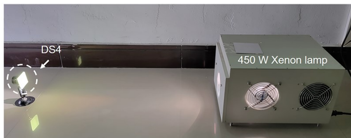
Fig. S15 (a) Photographs of DS4 irradiated by a Xenon lamp during photostability test. (b) The Xenon lamp spectrum.
