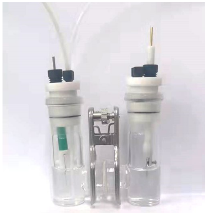
Fig. S22. Photo of in-situ electrochemical gas chromatography device.
