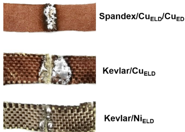
Figure S13. Control groups, Spandex/Cu ELD /Cu ED , Kevlar/Cu ELD (with 1.6- \mu m thickness of metal layer), and Kevlar/Ni ELD (with 0.6- \mu m thickness of metal layer) failed in the welding process with solder materials.
