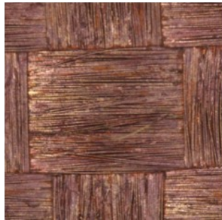
Figure S8. Optical microscope images of metallized Kevlar fabrics after cyclic attach–detach test.
