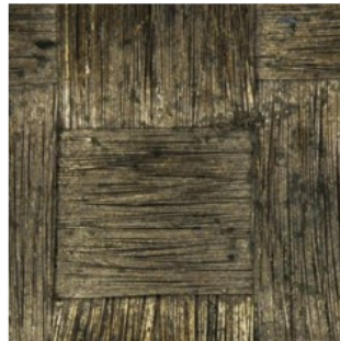
Figure S8. Optical microscope images of metallized Kevlar fabrics after cyclic attach–detach test.
