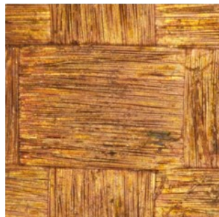
Figure S9. Optical microscope images of metallized Kevlar fabrics after simulated washing test.
