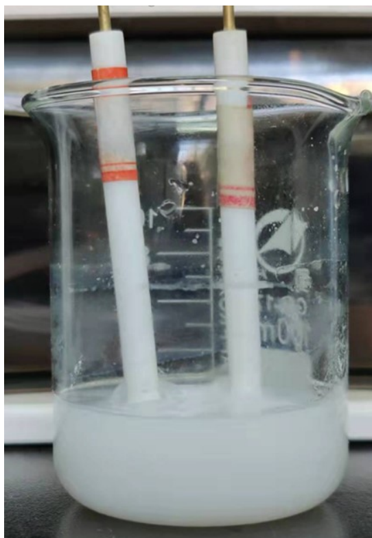
Figure S31 The optical image of the solid-state supercapacitor (OCC//CC supercapacitor based on PINE). The solid-state supercapacitor is in-situ fabricated by immersing OCC and CC electrodes into the precursor solution of PINE, in which OCC and CC are sandwiched with the white PTFE electrode clips. And cycled for 1000 cycles with the voltage window of 0~2.1 V at a current density of 18 \text{ mA cm}^{-2} . The area of CC and OCC is 1 \text{ cm}^2 . The supernatant has been poured out.
