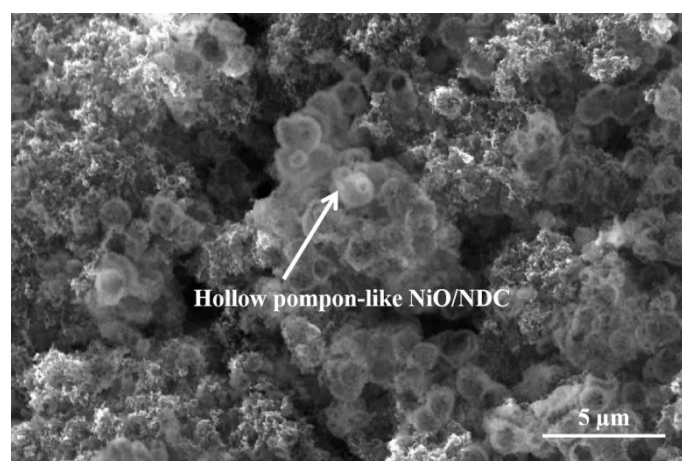
Fig. S19. SEM image of hollow pompon-like NiO/NDC after 100 cycles at current density of 0.5 C.
