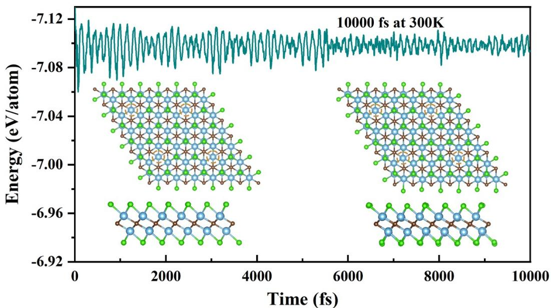
**Fig. S19** AIMD simulation of  $\text{Ti}_2\text{CCl}_2$  MXene with Cl vacancies. The inserts illustrate the initial and final (10000 fs) atomic structures shown in the top and side view. The orange dotted circles represent the Cl vacancies.
