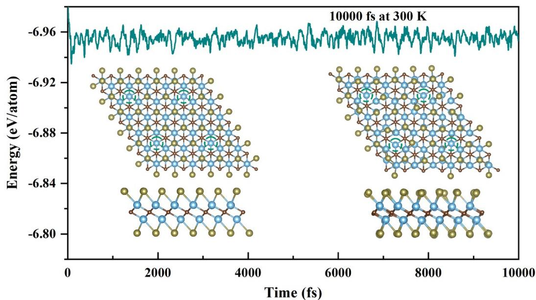
**Fig. S22** AIMD simulation of  $\text{Ti}_2\text{CTe}_2$  MXene with Te vacancies. The inserts illustrate the initial and final (10000 fs) atomic structures shown in the top and side view. The green dotted circles represent the Te vacancies.
