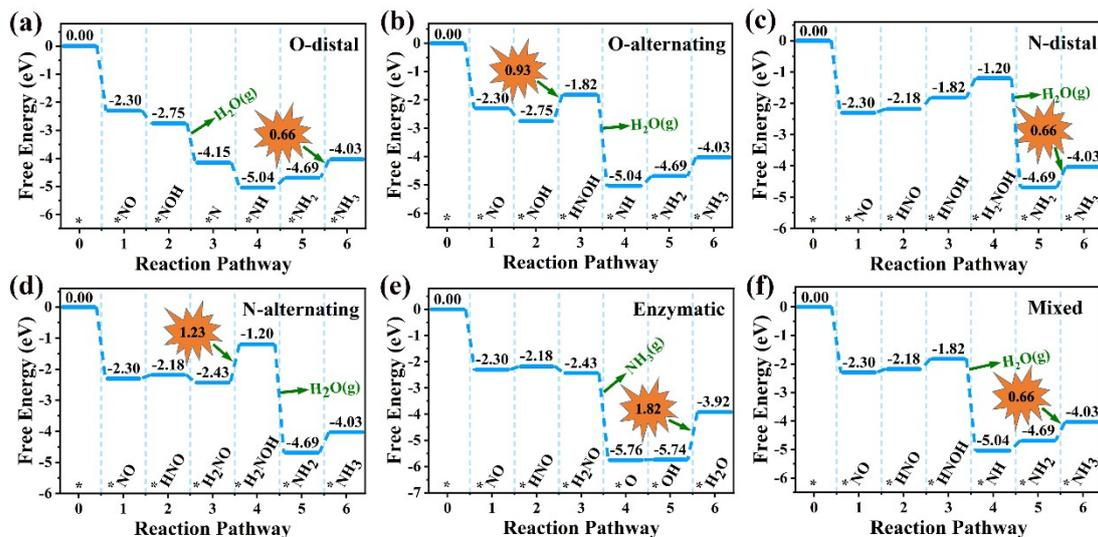
**Fig. S8** NORR free energy diagrams of the considered pathways on  $\text{Ti}_2\text{CCl}_2$  MXene. The applied potential is zero.
