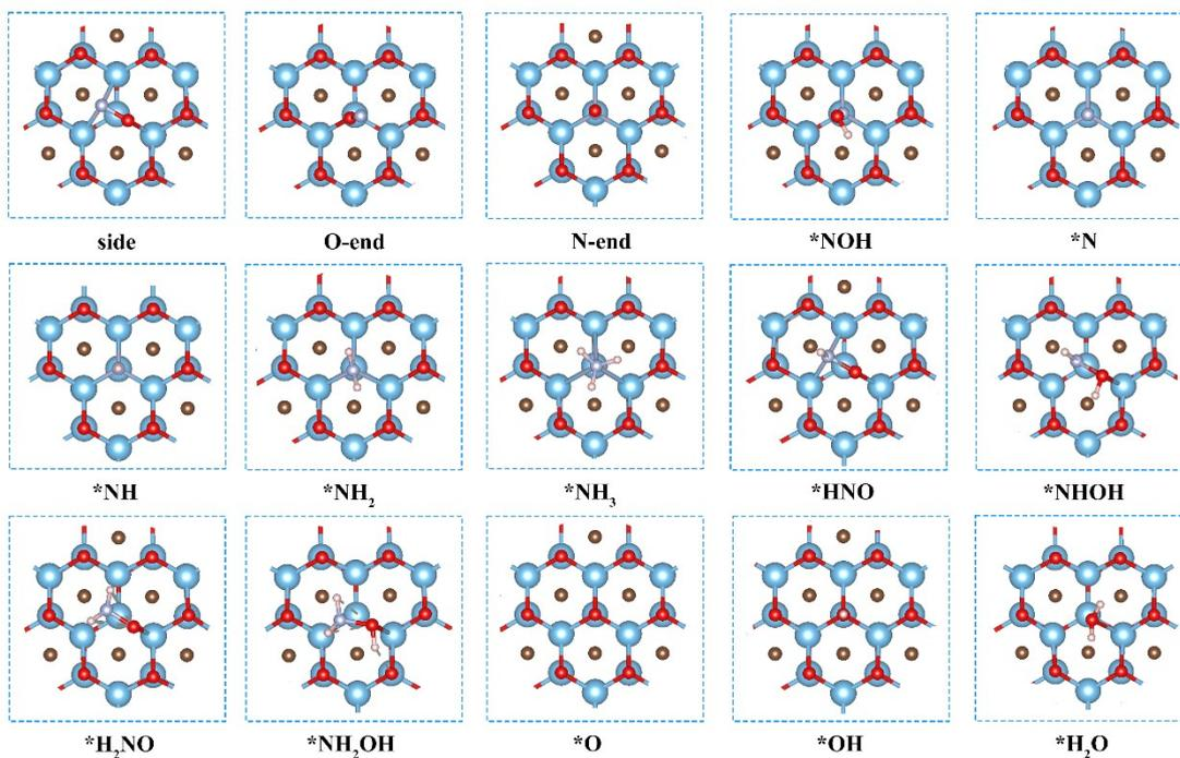
**Fig. S4** The optimized configurations of all NORR intermediates on  $\text{Ti}_2\text{CO}_2$  MXenes.
