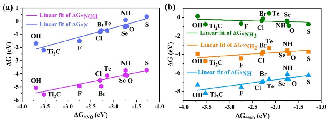
**Fig. S16** Linear scaling relations between the adsorption energies of involved intermediates of the most favorable pathway and the adsorption energy of NO ( $\Delta G_{*NO}$ ).
