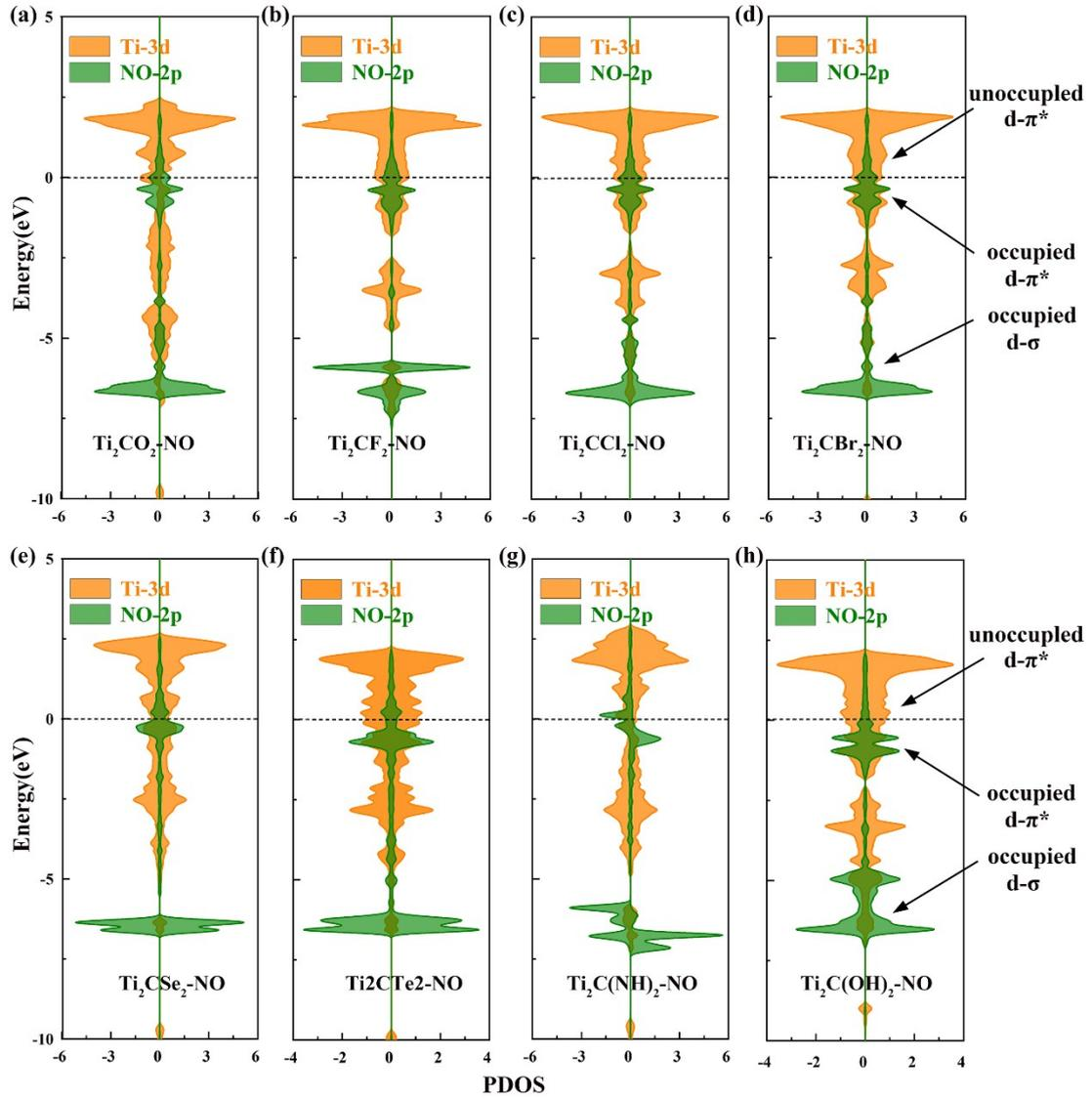
**Fig. S1** Partial density of states (PDOS) of the interaction between Ti-3d and NO-2p orbitals on NO absorbed functionalized  $Ti_2CT_2$  MXenes ( $T=O, F, Cl, Br, Se, Te, NH, OH$ ). The Fermi level is set to be 0 eV.
