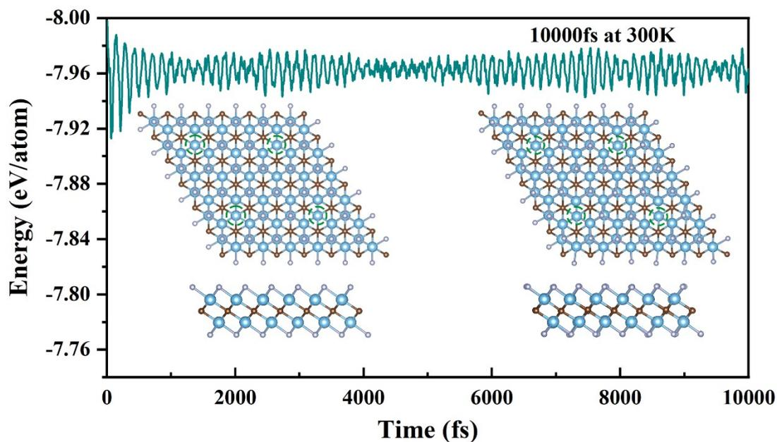
**Fig. S18** AIMD simulation of  $\text{Ti}_2\text{CF}_2$  MXene with F vacancies. The inserts illustrate the initial and final (10000 fs) atomic structures shown in the top and side view. The green dotted circles represent the F vacancies.
