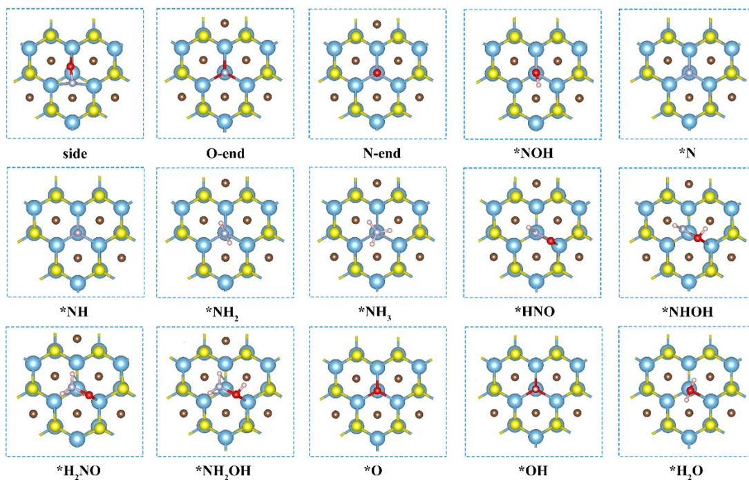
**Fig. S3** The optimized configurations of all NORR intermediates on Ti<sub>2</sub>CS<sub>2</sub> MXenes.
