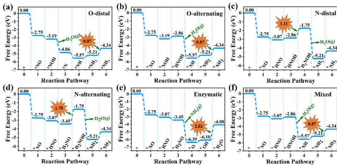
**Fig. S7** NORR free energy diagrams of the considered pathways on  $\text{Ti}_2\text{CF}_2$  MXene. The applied potential is zero.
