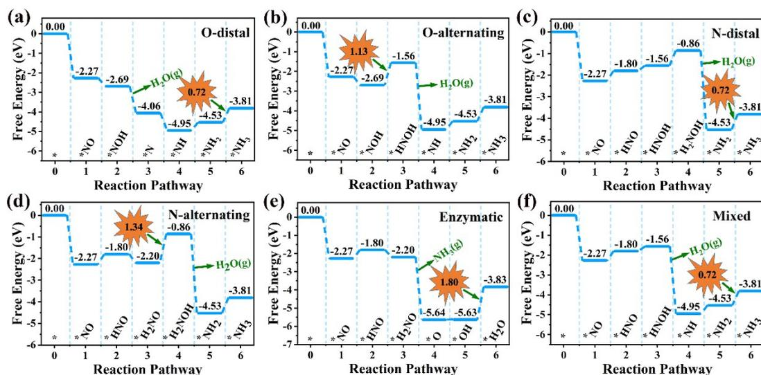
**Fig. S9** NORR free energy diagrams of the considered pathways on  $\text{Ti}_2\text{CBr}_2$  MXene. The applied potential is zero.
