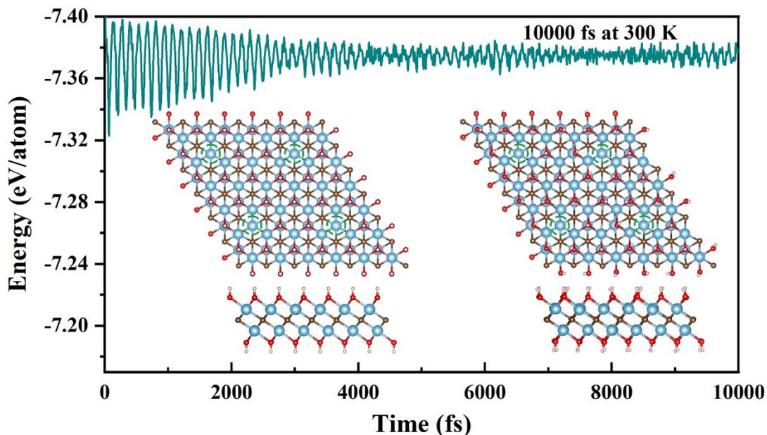
**Fig. S24** AIMD simulation of  $\text{Ti}_2\text{C}(\text{OH})_2$  MXene with OH vacancies. The inserts illustrate the initial and final (10000 fs) atomic structures shown in the top and side view. The green dotted circles represent the OH vacancies.
