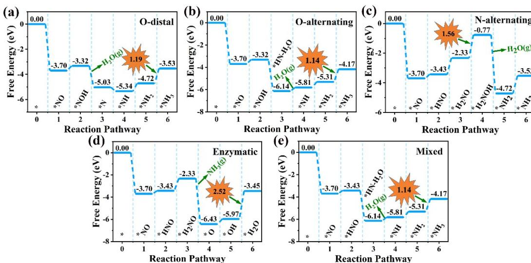
**Fig. S13** NORR free energy diagrams of the considered pathways on  $\text{Ti}_2\text{C}(\text{OH})_2$  MXene. The applied potential is zero.
