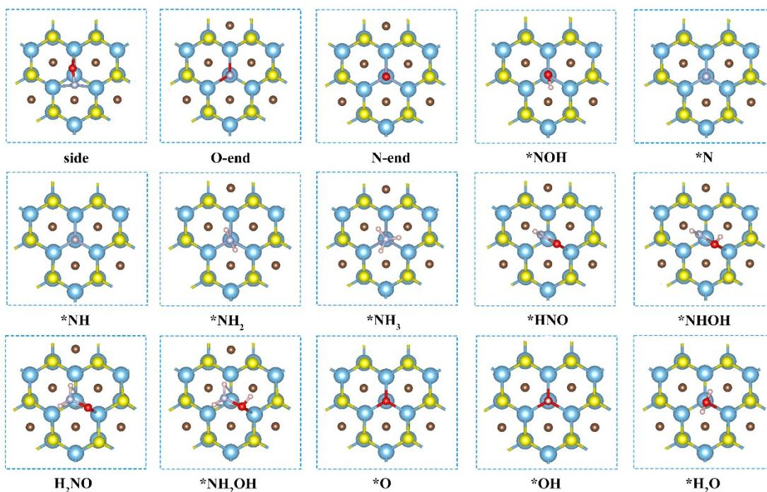
**Fig. S14** The optimized configurations of all NORR intermediates on  $\text{Ti}_2\text{CS}_2$  MXene with solvent effect.
