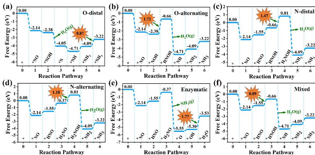
**Fig. S11** NORR free energy diagrams of the considered pathways on  $\text{Ti}_2\text{CTe}_2$  MXene. The applied potential is zero
