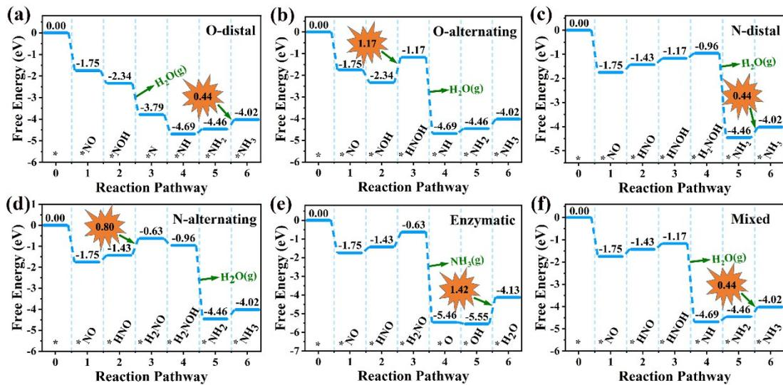
**Fig. S10** NORR free energy diagrams of the considered pathways on  $\text{Ti}_2\text{CSe}_2$  MXene. The applied potential is zero.
