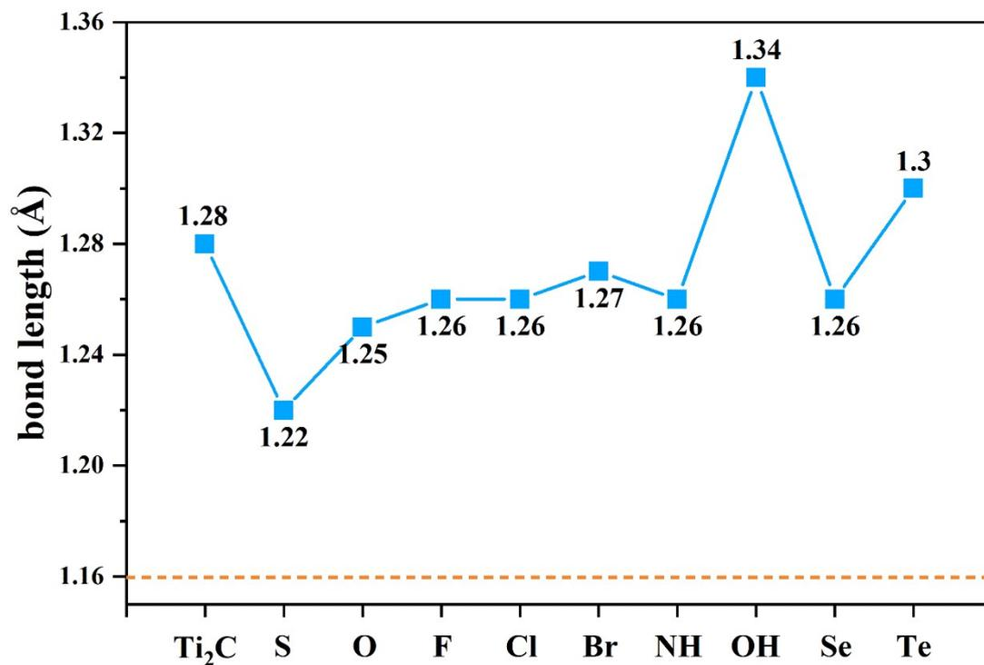
**Fig. S2** N-O bond length (Å) for NO adsorbed on bare Ti<sub>2</sub>C MXene and functionalized Ti<sub>2</sub>CT<sub>2</sub> MXenes. The orange dashed line represents N-O bond length of free NO gas molecule.
