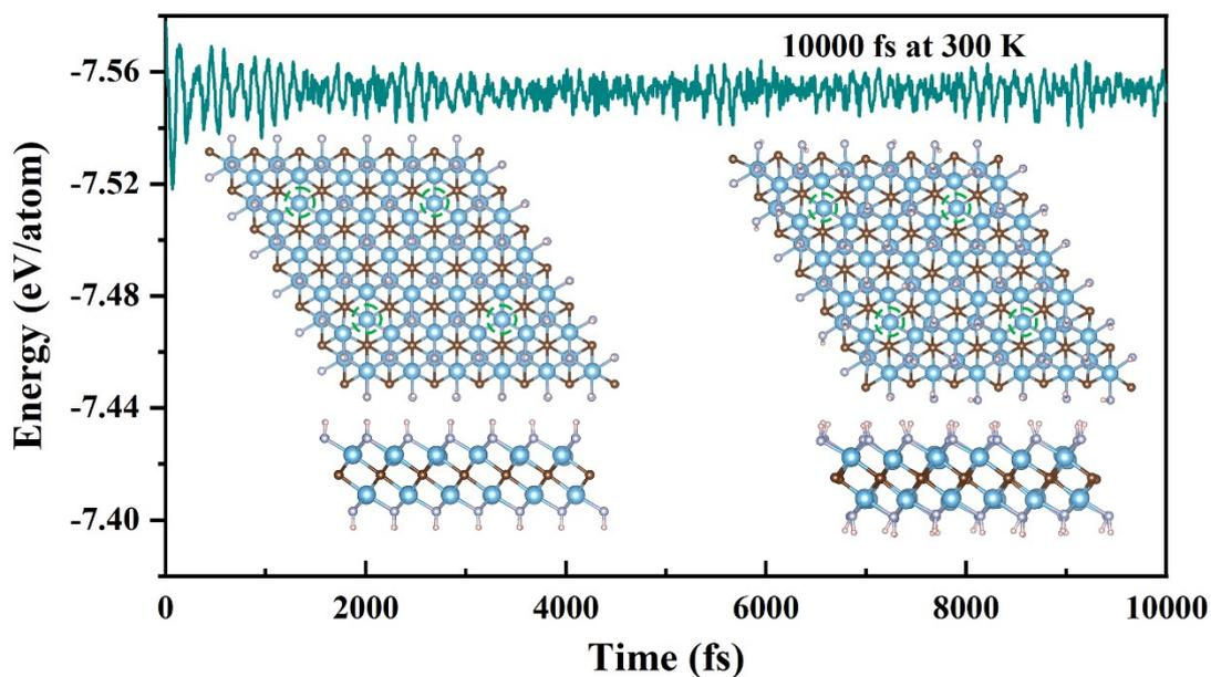
**Fig. S23** AIMD simulation of  $\text{Ti}_2\text{C}(\text{NH})_2$  MXene with NH vacancies. The inserts illustrate the initial and final (10000 fs) atomic structures shown in the top and side view. The green dotted circles represent the NH vacancies.
