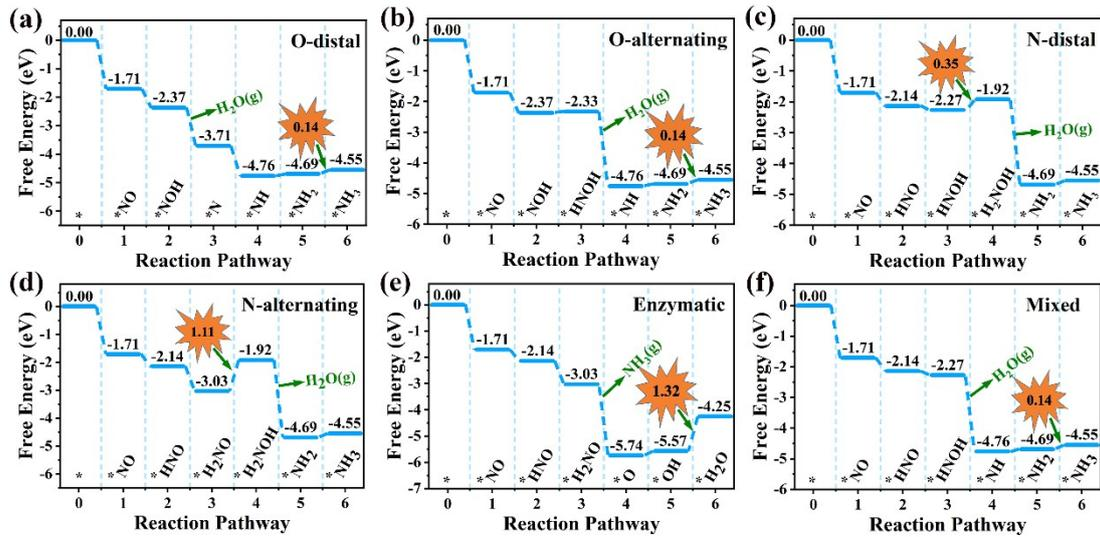
**Fig. S6** NORR free energy diagrams of the considered pathways on  $\text{Ti}_2\text{CO}_2$  MXene. The applied potential is zero.
