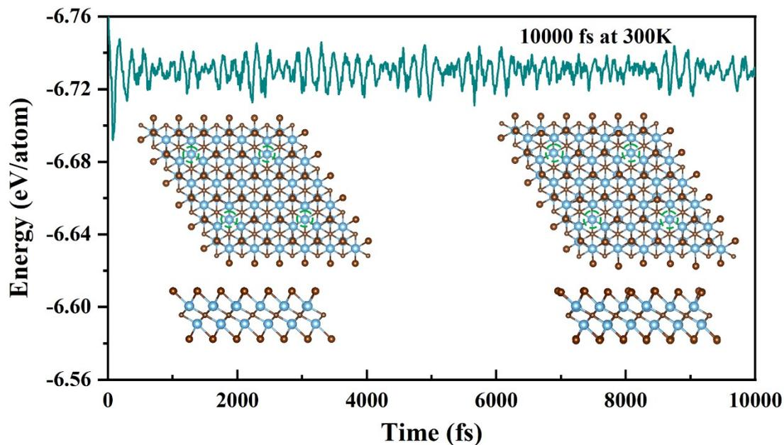
**Fig. S20** AIMD simulation of  $\text{Ti}_2\text{CBr}_2$  MXene with Br vacancies. The inserts illustrate the initial and final (10000 fs) atomic structures shown in the top and side view. The green dotted circles represent the Br vacancies.
