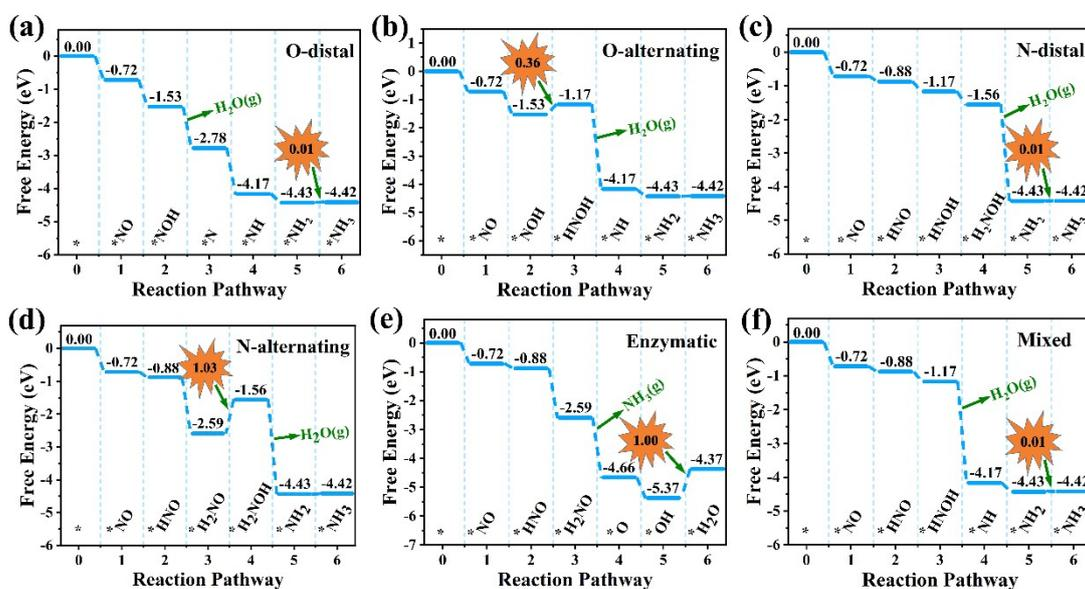
**Fig. S15** NORR free energy diagrams of the considered pathways on  $\text{Ti}_2\text{CS}_2$  MXene with solvent effect. The applied potential is zero.
