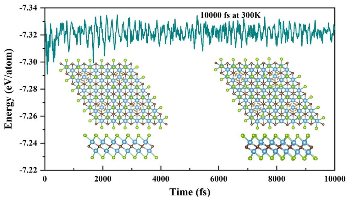
**Fig. S21** AIMD simulation of  $\text{Ti}_2\text{CSe}_2$  MXene with Se vacancies. The inserts illustrate the initial and final (10000 fs) atomic structures shown in the top and side view. The orange dotted circles represent the Se vacancies.
