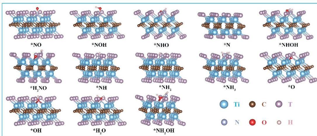
**Fig. S5** The optimized configurations of all NORR intermediates on functionalized  $\text{Ti}_2\text{CT}_2$  MXenes.
