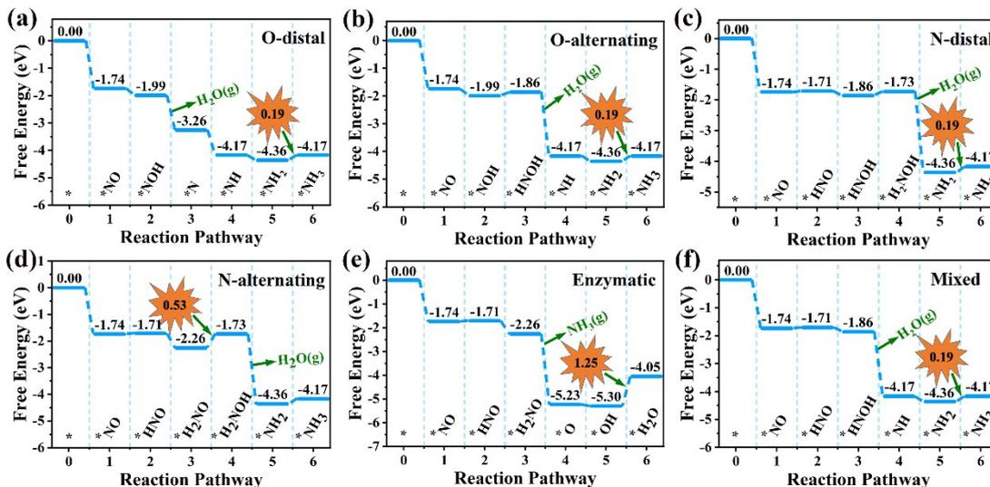
**Fig. S12** NORR free energy diagrams of the considered pathways on  $\text{Ti}_2\text{C}(\text{NH}_2)$  MXene. The applied potential is zero.
