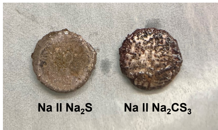
Figure S8. Optical photograph of Na-metal anodes after 20 cycles from the Na || Na 2 S (left) and Na || Na 2 CS 3 (right) cells.
