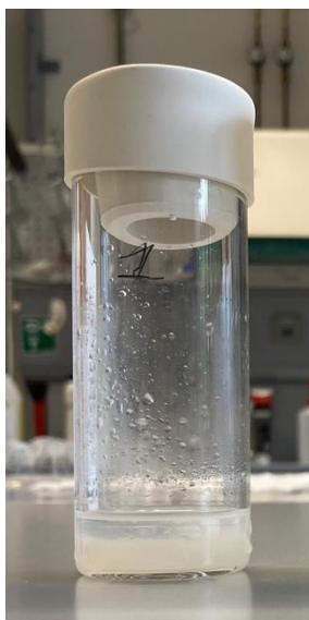
Figure S19. Photocatalytic tests. Photographs of biphasic system composed of 5 mL 1-octanol and 5 mL 1.0 \text{ mol L}^{-1} HCl with suspended HMDS photocatalyst after irradiation for 72 h with LED 406 nm ( 4.2 \text{ mW cm}^{-2} ), 22 \text{ }^\circ\text{C} , \text{O}_2 1 atm.
