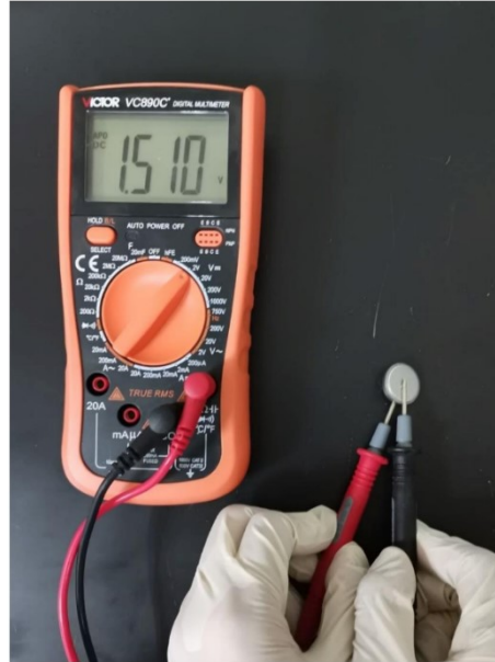
Fig. S23 Digital image of the button ZAB displaying an open circuit voltage of 1.51 V.
