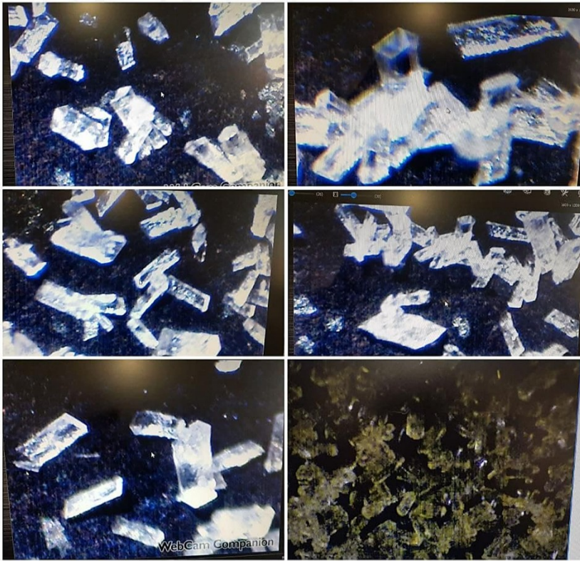
Figure S1. The optical images taken by an optical microscope from the as-prepared ZHO on the FGF surface
