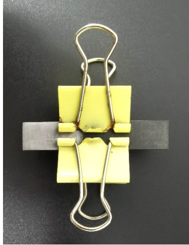
Figure S15. The bonding process of PSA under gently pressing by dovetail clip.
