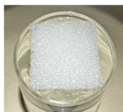
Figure S3. A white foam with area of 3 \times 3 \text{ cm}^2 is selected to subtract out the effect of exposed area in the evaporation device.
