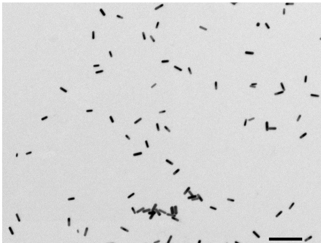
Figure S12. Low magnification images of (A) GNR@2 in PBS and (B) GNR@2-K in MilliQ water. Scale bar = 200 nm. 0.5% uranyl acetate staining was used.
