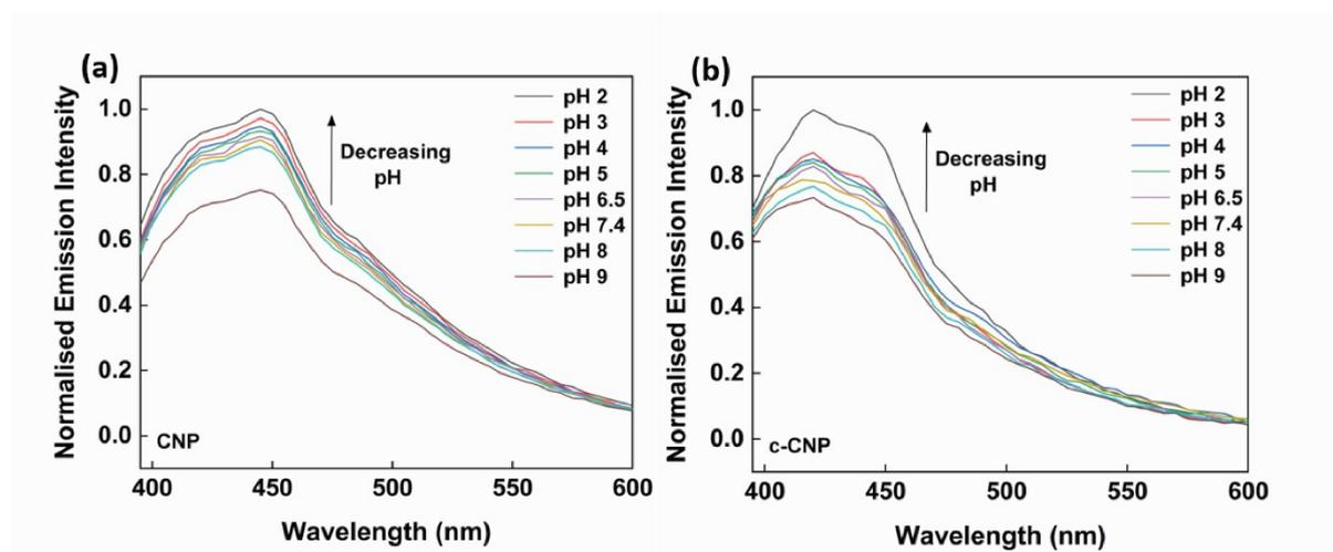
**Fig S5:** Emission spectra ( $\lambda_{ex}$  = 365 nm) for (a) CNP and (b) c-CNP in pH buffer solutions ranging from pH 2 to pH 9 indicating that fluorescence intensity reduces as pH value increases.
