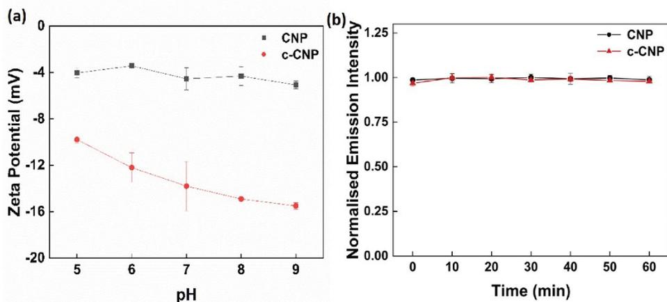
**Fig S4:** (a) Zeta potential curves for CNP (black solid line) and c-CNP (red solid line) showing change in zeta potential values with varying pH (pH 5 to pH 9). (b) Plot showing photostability of CNP and c-CNP ( $\lambda_{ex}$  = 365 nm and  $\lambda_{em}$  = 450 nm) exposed to UV lamp for 60 min.
