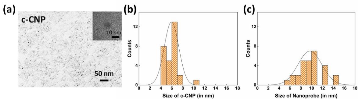
**Fig S1:** (a) Transmission electron microscope image of c-CNP showing nanoparticles with spherical morphology. The inset shows HRTEM image of the c-CNP; Size distribution histograms for (b) c-CNP and (c) Nanoprobes.
