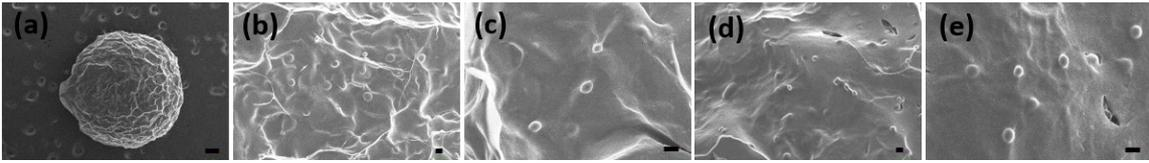
**Fig S13:** Scanning electron micrographs of **(a)** blank microscaffolds (Scale bar: 300  $\mu\text{m}$ ); and microscaffolds with U2OS cells cultured for 24 hr **(b)**, **(c)** without and **(d)**, **(e)** with c-CNP. (Scale bar: 20  $\mu\text{m}$ )
