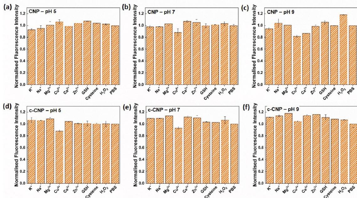
**Fig S9:** Normalised fluorescence intensity of CNP (a-c) and c-CNP (d-f) at pH 5, 7 and 9 in presence of various metal ions, biothiols and ROS.
