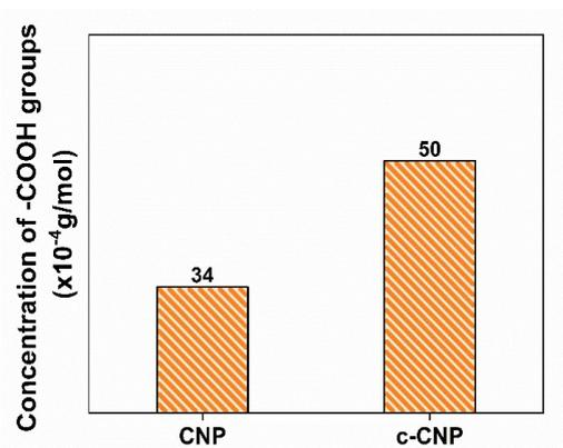
**Fig S3:** Bar graph showing increase in concentration of -COOH functional groups on nanoparticles' surface post carboxylation as calculated by Boehm's titration method.
