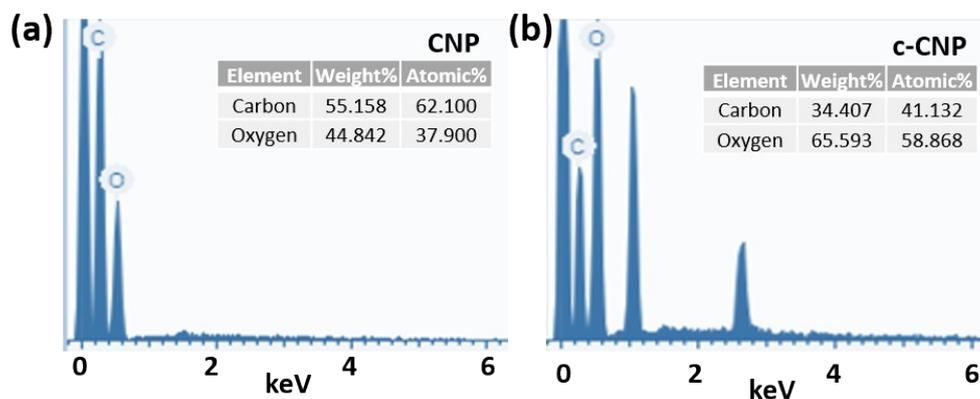
**Fig S2:** Elemental analysis for (a) CNP and (b) c-CNP using Energy dispersive X-ray Analysis
