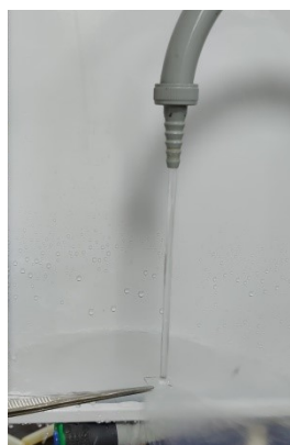
Figure S35 Scouring test of coating under the faucet (glass substrate).
