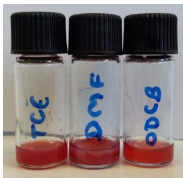
Figure S3. C 3 Pyr/C 3 NDI (1:1) organogels obtained in different solvents (TCE, DMF, oDCB).
