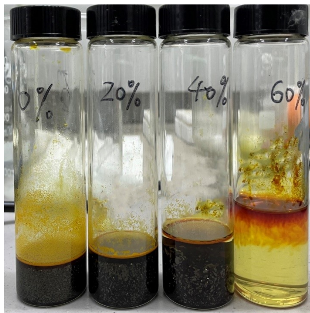
Fig. S2 Pre-test of TEA 2 SnI 4 SCs. The vial marked means the volume ratio of ethanol versus HI. When ethanol was added up to 60 %, there were no product.
