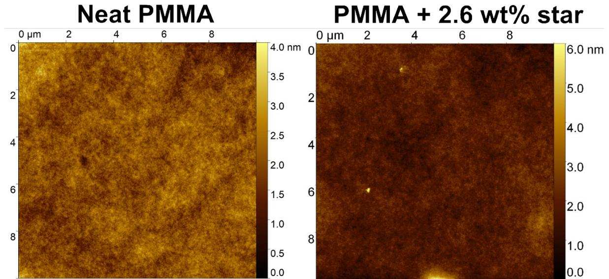
**Figure S2.** AFM height images (10  $\mu\text{m}$  x 10  $\mu\text{m}$ ) of neat PMMA dielectric layers (left) and PMMA layers with ca. 2.6 wt % of polymer star without the  $\text{TiO}_2$  (right).
