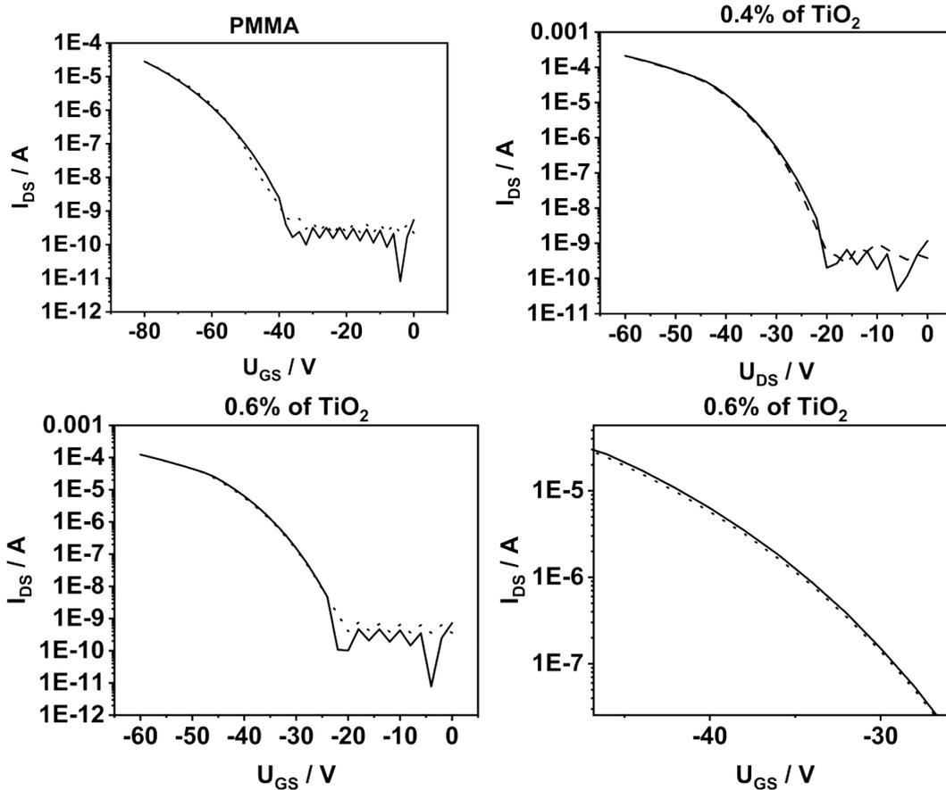
**Figure S5.** Transfer characteristics of the OFETs with C8-BTBT semiconductor layer nominally ca. 20 nm thick, and with dielectric layer made of neat PMMA or PMMA containing 0.4 % or 0.6% of TiO<sub>2</sub>. Straight lines are forward and dotted lines are backward sweeps; the last plot is a magnification of the curve measured for the sample with PMMA containing 0.6% TiO<sub>2</sub>.
