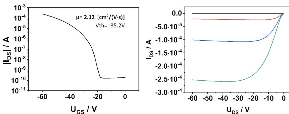
**Figure S3.** Transfer and output characteristics of the OFETs prepared on Si/SiO<sub>2</sub> substrates; the C8-BTBT semiconductor layer was nominally ca. 50 nm thick.
