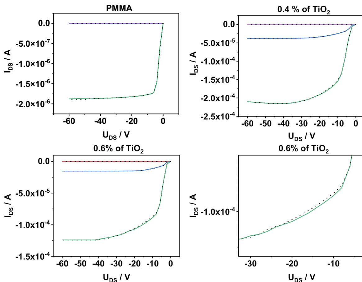
**Figure S4.** Output characteristics of the OFETs with C8-BTBT semiconductor layer nominally ca. 20 nm thick and with dielectric layer made of neat PMMA or PMMA containing 0.4 % or 0.6% of  $TiO_2$ . Straight lines are forward and dotted lines are backward sweeps; the last plot is a magnification of the curve measured for the sample with PMMA containing 0.6%  $TiO_2$ .
