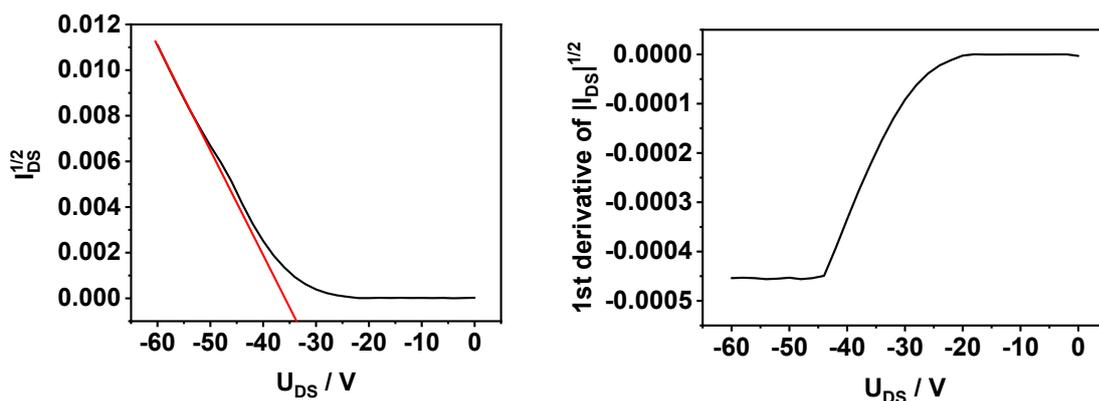
**Figure S6.** Transfer characteristic of the OFETs with C8-BTBT semiconductor layer nominally ca 20 nm thick, and with dielectric layer made of PMMA containing 0.6% TiO<sub>2</sub>. The red line is the fitted line used to determine the threshold voltage; 1<sup>st</sup> derivative of the transfer curve. The fitted range in the transfer curve corresponds to the voltage range when the first derivative is constant.
