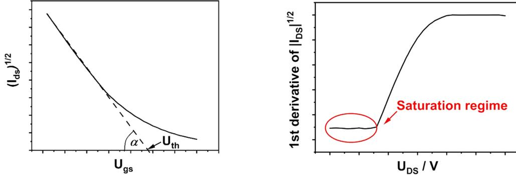
**Figure S1.** OFET transfer characteristics with a straight line intersecting the  $U_{gs}$  axis at  $U_{th}$  at the  $\alpha$  angle fitted to the linear region of the curve (saturation regime of the OFET) and 1<sup>st</sup> derivative of this curve with marked range of the constant value corresponding to saturation regime of the OFET.
