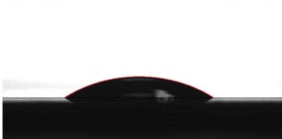
Fig. S4. Water contact angle images of the (a) AX and (b) BG films.
