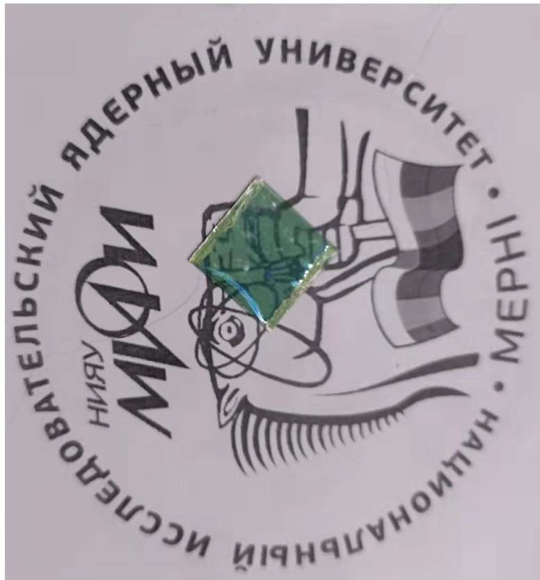
Figure S4. Optical photograph of PFP flexible pressure sensor placed on patterned paper.
